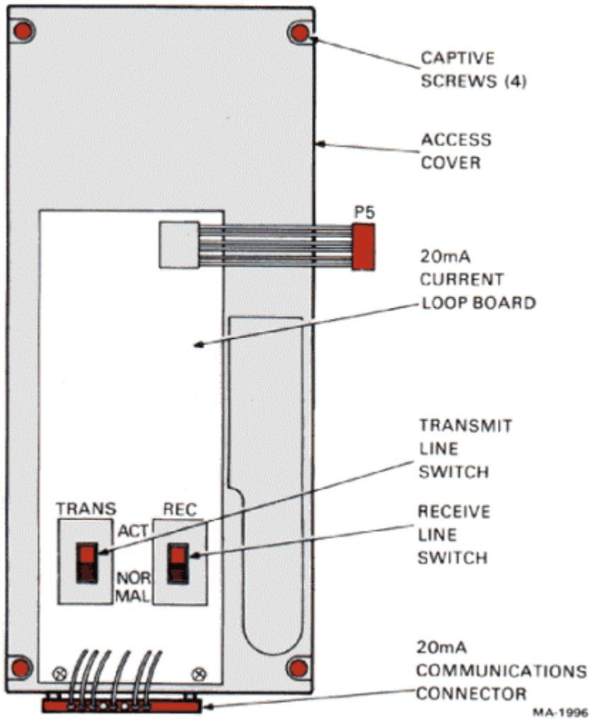
Figure 4-4 Terminal Controller Board
